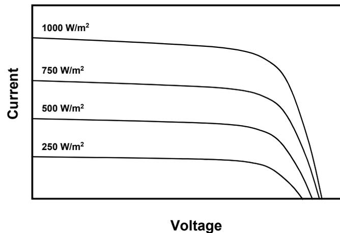
**Figure 4. IV curve response to irradiance, constant temperature.**
