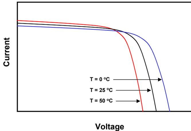
**Figure 5. I-V curve response to cell temperature.**
