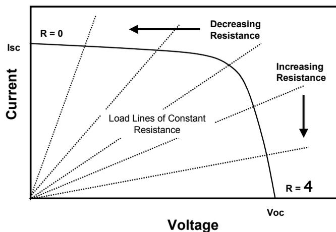
**Figure 3. I-V curve with load lines of constant resistance.**
